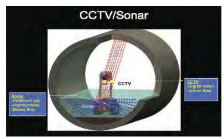
Sonar and CCTV technologies can be used together to evaluate the condition of a collection system.
