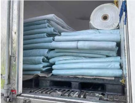
Liner materials are designed and manufactured for each individual pressure pipe installation, and shipped to the site in refrigerated trucks
