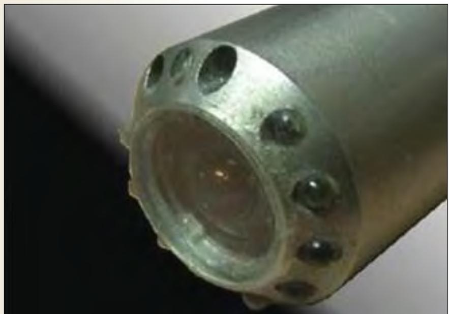
Figure 1. View of the CCTV Camera of the LDS1000
