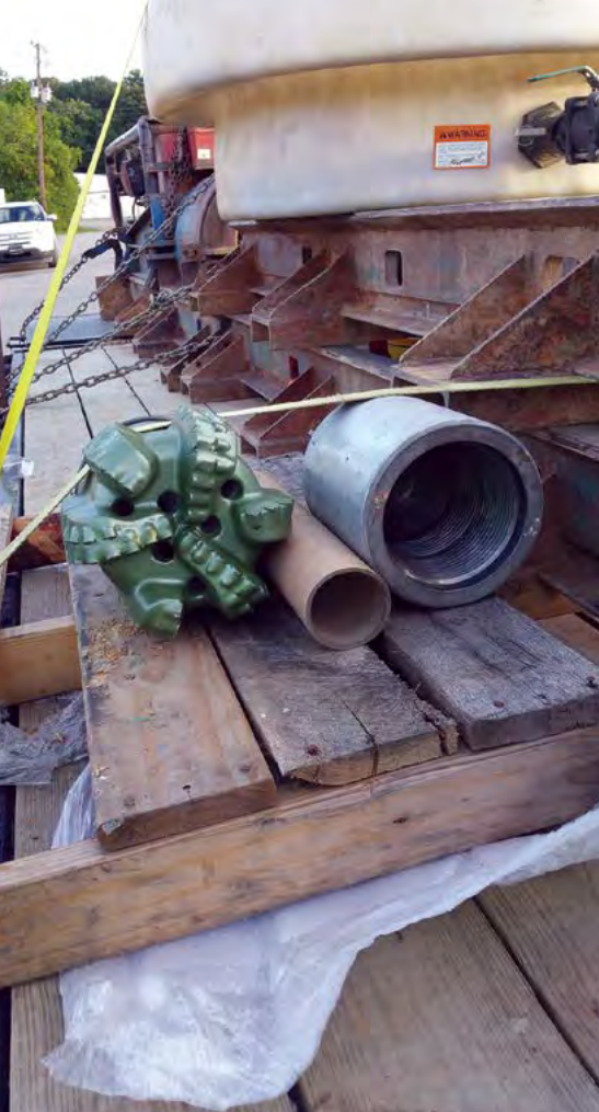
US Crossings ordered a 9-7/8 inch PDC bit out of Texas and had it hot-shotted over night to the jobsite.
