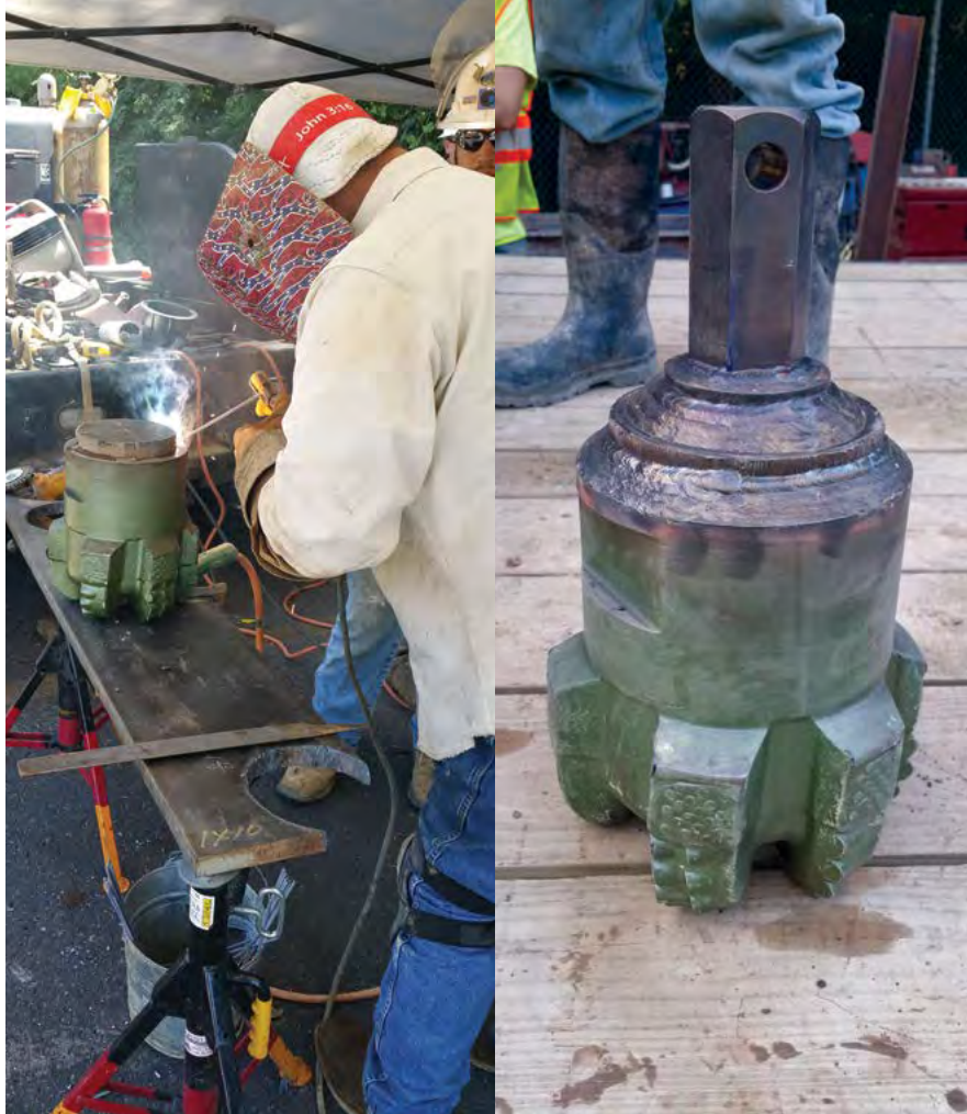
The 5-1/2 inch full hole threads were cut off the PDC bit and converted over to 2-1/4 inch hex to fit the auger bore rig.
