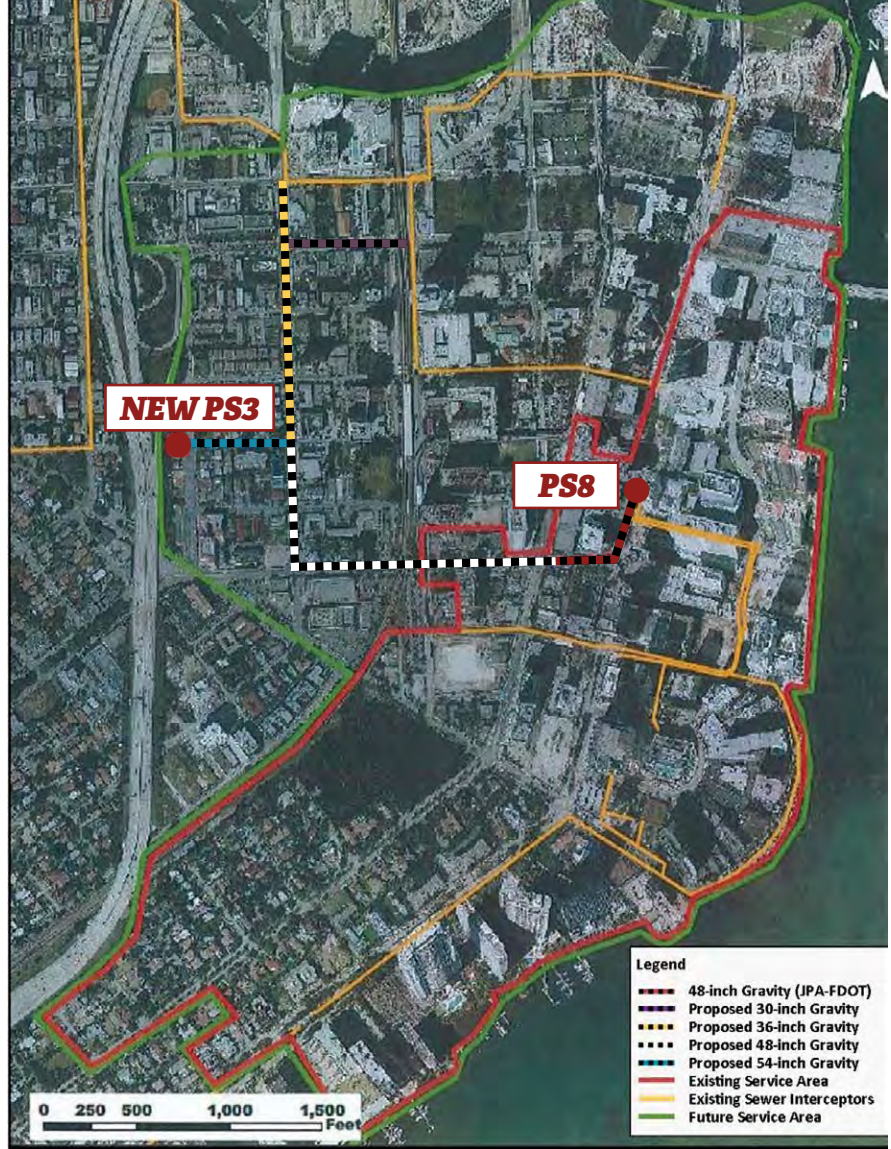
Located in densely populated downtown Miami, the new wastewater conveyance system required innovative solutions. A new gravity sewer interceptor was needed to reroute flows from existing pump station PS8 to new pump station PS3
