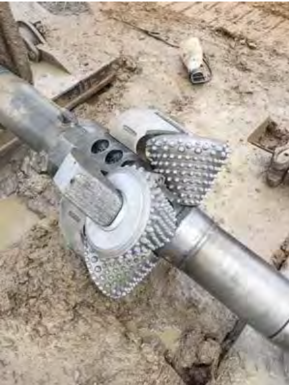
V10 Viper. Pilot hole straight to 32 inches. 22,000 PSI Rock (104 hours)
