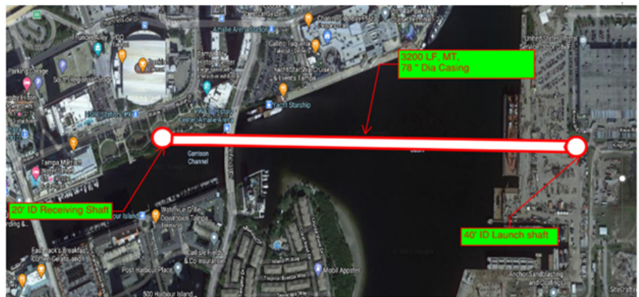
Figure 1: Location and dimensions of microtunnel and shafts between the Port of Tampa (right) and downtown Tampa (left). Image provided by Primoris Services Corp
